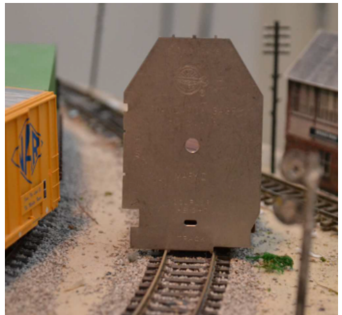
Fig 7 Checking the Rail Gauge with the NMRA track gauge. The whole profile of the gauge is to allow for the overhang of rolling stock clearing tunnel mouths, buildings and signals. It is a lifetime investment as an aid to better track laying.
