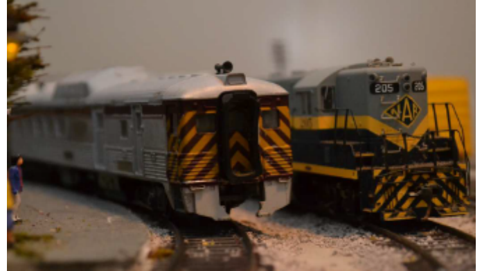
Fig 12 Northern Alberta Railways 205 arriving for a cross with an Eastbound RDC3. The angle of super elevation gives an effect I am happy with although I have seen higher camber levels
