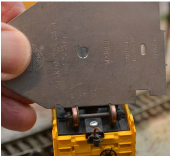
Fig 8 Checking the gauge of the wheels in situ. These notches are set for the correct back to back spacing of wheels.
