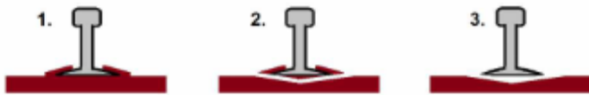
Fig 4 This is showing undercutting the rail so that rail joiners can be inserted.
