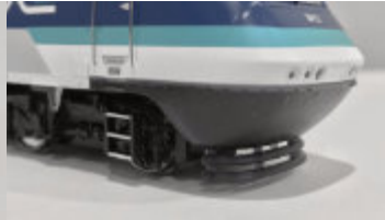
Twin Bar & Catcherless Pilot for early XPT Powercars
