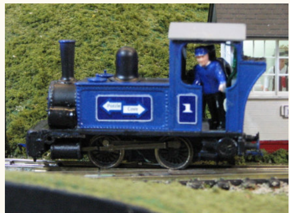
Fig. 14 Engine number 1. The capacitors are disguised as an air tank under the cab floor and level with the rear buffer and an oil tank below the stack in front of the water tank.
