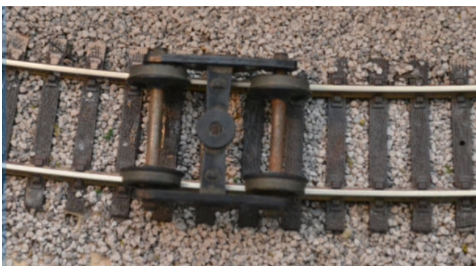
Fig.8 It may be difficult to pick up at first glance but the wheels to the right are not central on the axles and slightly out of gauge. The truck sides are then not travelling squarely on the rails, and that becomes a potential problem.
