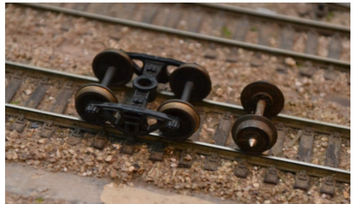
Fig. 1 An older MDC/Roundhouse truck/bogie fitted with North Yard RP25 metal wheels alongside a deep flanged wheel set. Note the difference with the appearance of the flanges. The operation of the truck is a lot smoother than this example of a European wheel. The sharp edges will pick at faults.
