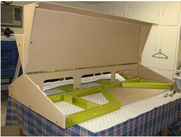
Fig. 5 Complete with hinging, the box is taking shape on the frame.
