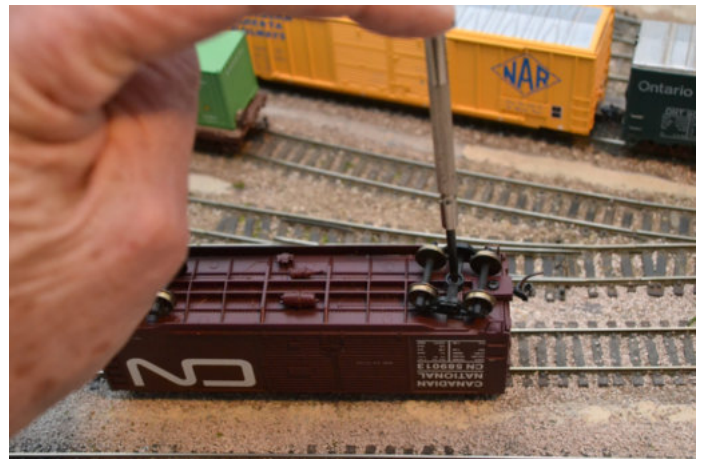
Fig.7 Loosening a truck on an Athearn Box Car. A Quarter to Half turn should ease the movement of the truck considerably.
