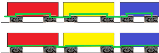
Fig. 10 The Green line is showing the transmission of force between truck mounted (upper) and body mounted couplers.
