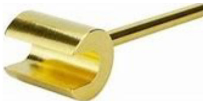
Fig.2 An Alternative Back to Back measuring tool. This tool could also be made using a thick metal or styrene block, accurately machined or filed to the back to back measurement.
