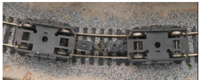
Fig. 9 These are passenger car trucks with the one on the right in “push” mode from the right hand side. With truck mounted couplers, there is very little performance difference in “pull” mode.
