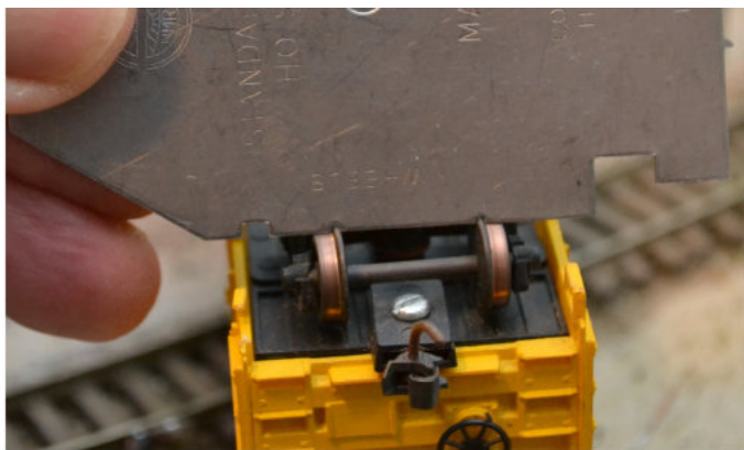
Fig. 6 Checking the gauge of the wheels in situ. The notches are set for the correct spacing of wheels and are the depth of the RP25 flange size.
