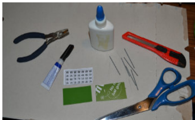
Fig. 6 The tools are simple enough for this exercise. Shown are the 40mm long pins, the speed board labels, plastic container lids from a yoghurt tub. The white glue is for the paper on the smooth side of the plastic while the mottled labelled side represents the casting effect. The labels once they are glued can be cut with ordinary scissors and trimmed if necessary with the snap blade knife.
