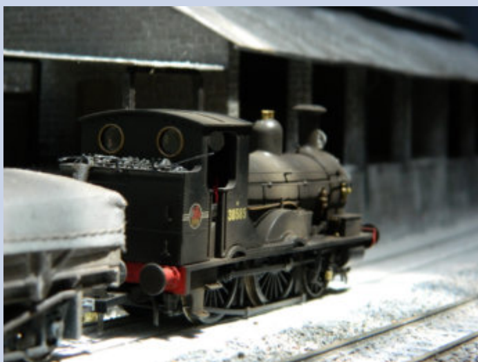
Fig. 13 A portrait of Beattie “well tank” 30585 at Carrgelyp clay dries. The clay is white which accounts for the colour across the track. I used a mix of casting plaster and white weathering powder. The loco itself has been detailed with the addition of a bucket (which they always seemed to carry) fire-irons, weathering and lump coal in the bunker.
