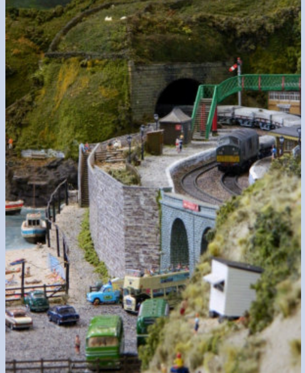
Fig. 21 A class 22 leads a train of four wheel china-clay wagons through the curves at Penhayle Bay station. The huge hillside beneath which the railway tunnels is just beyond the station. The Down starting signal is placed on the “wrong” side of the line to aid visibility in a prototypical manner.
