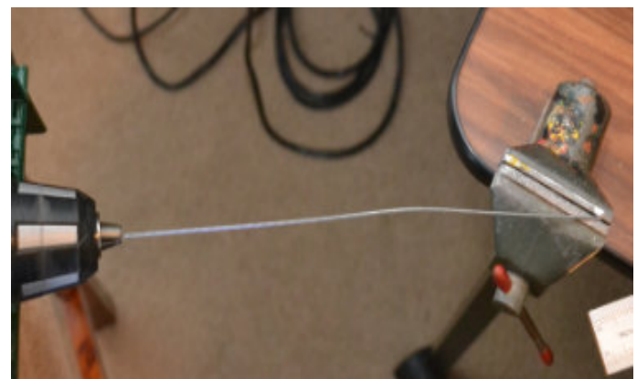
Fig. 4 Step 2. By holding the wire taut and spinning the power drill, you will work harden the wire and straighten it. It will not twist totally out of shape as you might think at first. Although this is a safe operation, please think safety and wear safety glasses.
